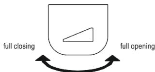
Fig. 4. The example adjustment of the air supply to the furnace
